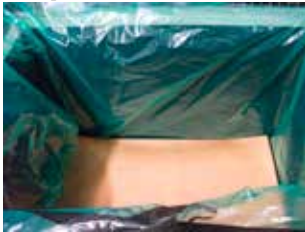
place Branorost paper on the new plastic lining
