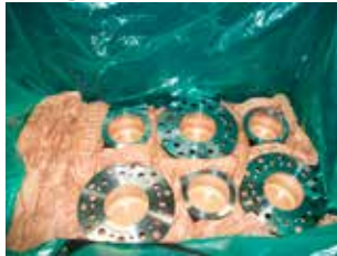
place soda kraft paper Natron Misch 80 g or Branorost 80 g for material padding
